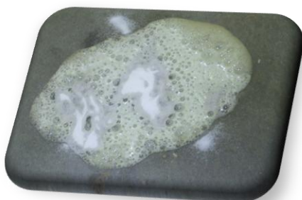
TYPICAL DRY NEUTRALIZER (Note the violent reaction)
