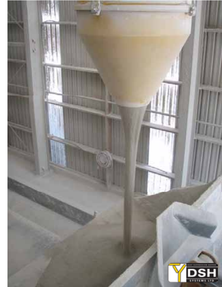
Converging powder stream rapidly thins. No dust emission from falling jet occurs.
